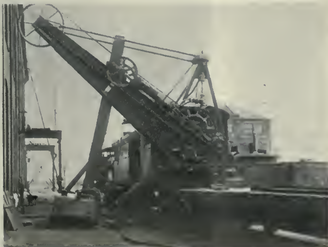
65-ton steam shovel purchased by the Canadian Government for the Canadian Overseas Railway Construction Corps.
